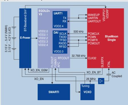
The BlueMoon™ Single is the perfect match for Bluetooth™ enabled handheld applications such as mobile phones, PDA and others, where board space, amount of external components and price are the dominating criteria. The block diagram provides an overview of a complete mobile phone system solution based on Infineon GSM/GPRS and Bluetooth™ solutions.
